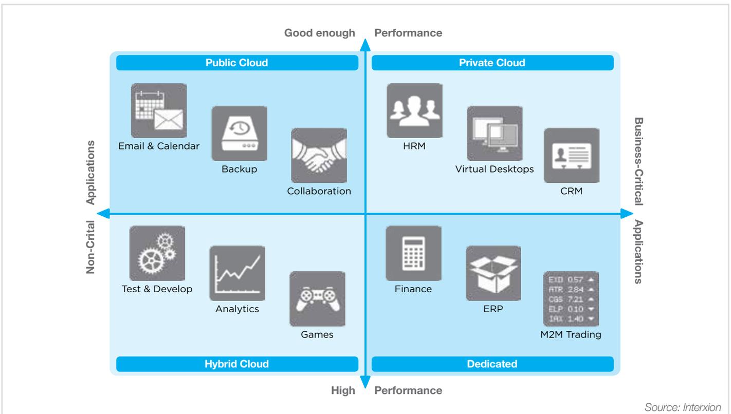
The diagram demonstrates how cloud, location, performance and applications can be brought together. General applications such as e-mail and collaboration are not high performance and can be placed on public cloud. At the other end of the spectrum are applications that are business-critical, highly sensitive and require high performance systems, such as ERP, finance and M2M trading. These are best run on dedicated systems where the business can provide security and risk analysis.
